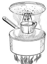
Distillation is an effective method of water purification.
